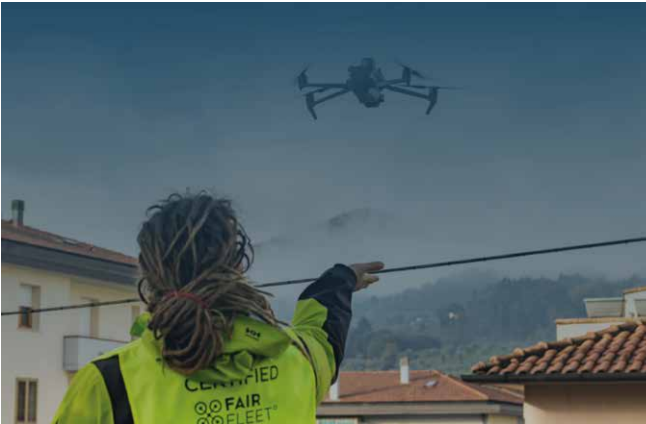
Above , Drone for inspecting facades and roofs equipped with technology for recognizing anomalies and malfunctions. Below , Inspection flight with drones controlled by a specialized operator.
